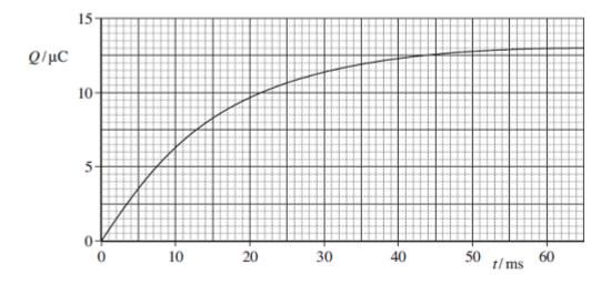
(b) (i) When the capacitor is fully charged, the charge stored is  $13.2 \ \mu$ C. The electromotive force (emf) of the battery is 6.0 V. Determine the capacitance of the capacitor.
