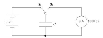
The switch is driven by a signal generator and oscillates between  $S_1$  and  $S_2$  with frequency *f*.
