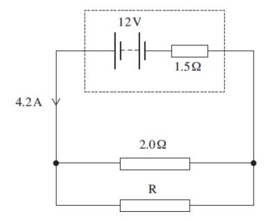
(a) (i) Show that the potential difference (pd) across the internal resistance is 6.3 V.
