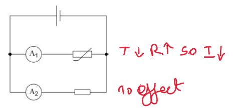
The cell has a constant electromotive force and negligible internal resistance. Readings from the two ammeters are taken.
