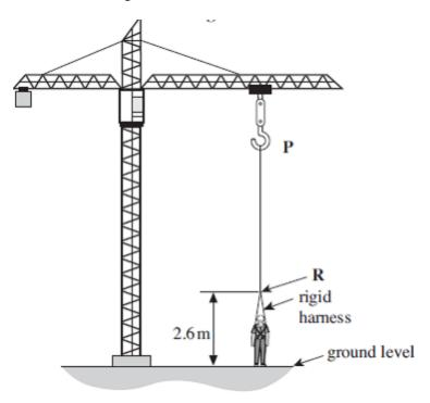
The rope has an unstretched length of 20 m. When stretched, the rope obeys Hooke's law and has a stiffness of 92  $Nm^{-1}$ . In the following questions ignore the mass of the rope.
