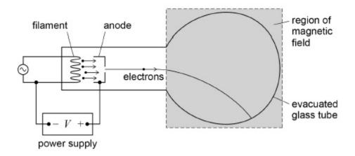
Electrons are emitted from the filament and accelerated by a potential difference between the filament and anode to produce a beam. The beam is deflected into a circular path by applying a magnetic field perpendicular to the plane of the diagram.
