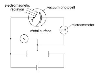
The potential divider is adjusted until the photocurrent is zero.
