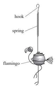
(a) The mass of the flamingo is 65 g. When the flamingo is suspended vertically the spring extends by 8.5 cm.
