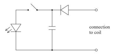
Once the torch has been shaken for a few minutes the switch is closed and the LED lights for a short while.
