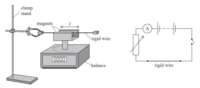
With the switch open, the balance was set to zero. When the switch was closed a current I in the circuit was recorded by the ammeter and the reading on the balance increased.
