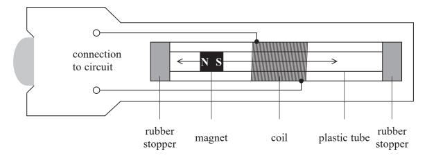
Each time the magnet moves through the coil a current pulse is generated. The coil is connected to a capacitor via a diode, as shown.
