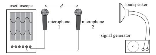
The microphones detect sound from the loudspeaker, converting it to an electrical signal. The signal is displayed on the oscilloscope screen.
