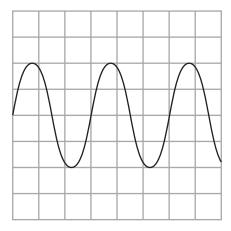
The time base of the oscilloscope was set to 0.20 ms div<sup>-1</sup>.
