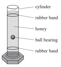
(a) The student placed rubber bands near the top and bottom of the cylinder. He started a stopwatch when the ball bearing passed the first band and stopped the stopwatch when the ball bearing passed the second band. He repeated this several times to determine a mean time.
