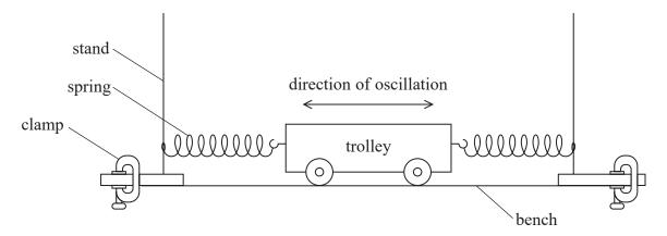
The student displaced the trolley from its equilibrium position. She then released the trolley and started a stopwatch. She stopped the stopwatch when the trolley had completed one oscillation.
