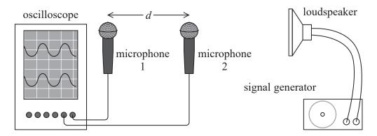
The microphones detect sound from the loudspeaker, converting it to an electrical signal. The signal is displayed on the oscilloscope screen.
