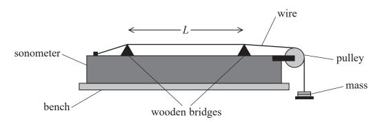
The student placed the base of a vibrating tuning fork in contact with the wire, at one of the bridges. This set the wire into oscillation. He adjusted the position of the other bridge until a single-loop standing wave was produced on the wire between the bridges.
