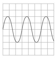
The time base of the oscilloscope was set to 0.20 ms div<sup>-1</sup>.
