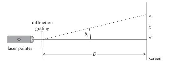
The distance between the first order maximum and the central maximum of the diffraction pattern was x. The distance between the diffraction grating and the screen was D.
