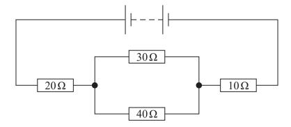
Calculate the total resistance of the resistors in the circuit.
