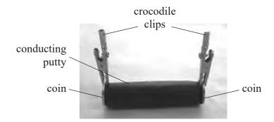
Determine the resistance of the cylinder of putty.
