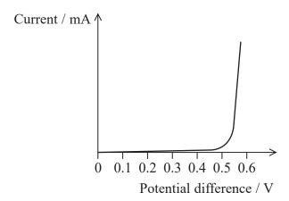
Describe how the student could adapt her method to plot the variation of current with potential difference for the diode in forward bias.
