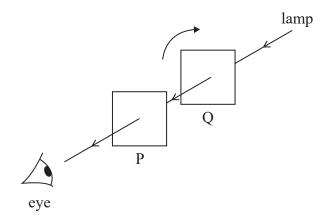
The lamp appears dark when viewed through P and Q. Q is rotated through 180°.
