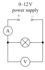
The student increased the output from the power supply from 0 V to 12 V in steps of 2 V. She recorded corresponding currents from the ammeter.
