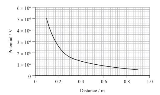
Air molecules will be ionised if the electric field strength exceeds  $3 \times 10^6 \, V \, m^{-1}$ .
