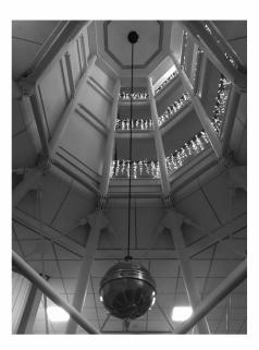
This is a pendulum that consists of a massive sphere, suspended by a long wire from a high ceiling. Over time the vertical plane through which the pendulum swings appears to rotate because of the rotation of the Earth.
