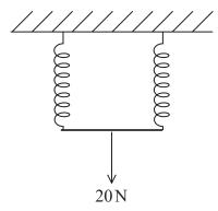
When a force of 20 N is applied, an extension of 8 cm is obtained.
