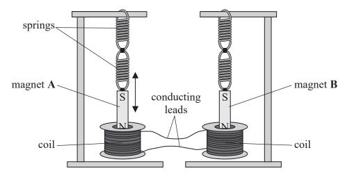
Magnet A is displaced so that it oscillates vertically. The North pole of magnet A moves into and out of the coil of wire with simple harmonic motion. As this motion continues, magnet B starts to oscillate. The amplitude of oscillation of magnet B increases over time.
