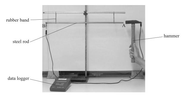
The rod is tapped at A with the hammer. A compression pulse travels to B and is reflected back. When the reflection reaches A the hammer loses contact with the rod. Whilst the hammer is in contact with the rod the output from a 5V supply is recorded by the data logger.
