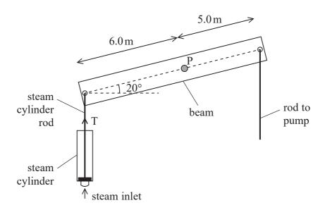
(a) The beam has a constant thickness and a mass of  $3.05 \times 10^4$  kg. The length of the beam is 11.0 m. The pivot P is positioned 6.0 m from the steam cylinder end of the beam.
