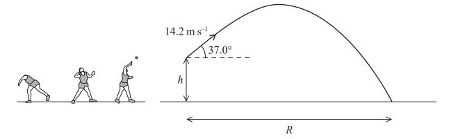
A shot is thrown from a height h above the ground with an initial velocity of 14.2 m s<sup>-1</sup> at an angle of 37.0° to the horizontal. The time it takes for the shot to reach the ground is 1.98 s.
