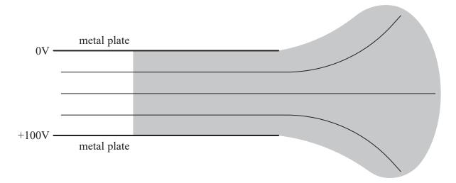
(a) Draw lines to represent the electric field in the shaded area.
