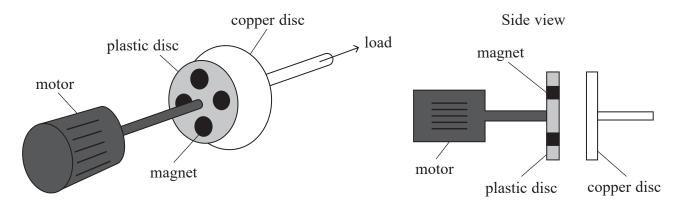
Several magnets are embedded in the plastic disc and it is rotated by the motor.
