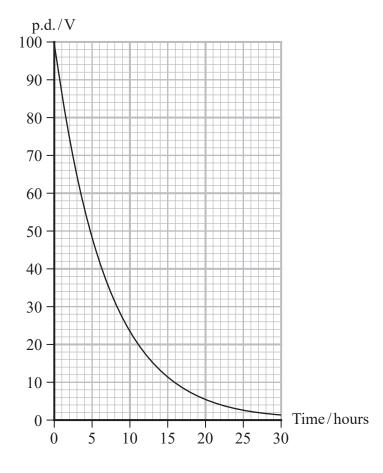
The insulator is a type of plastic and should have a resistivity greater than  $10^{14}\Omega m$ . Deduce whether the plastic used in this capacitor has a resistivity greater than this value.  $A = 5.6 \times 10^{-3} \,\mathrm{m}^2$  $d = 0.6 \times 10^{-6} \,\mathrm{m}$ **(5)** (Total for Question 13 = 9 marks)
