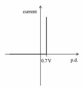
(a) Describe how the current through this diode varies for positive p.d.s and negative p.d.s.
