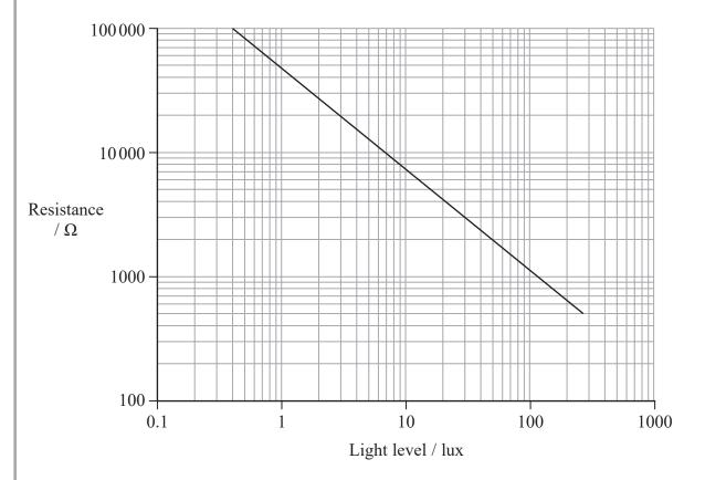
The transistor switches on when the potential difference across the input increases above 0.7 V. This should happen as the light level reaching the LDR increases above 30 lux.
