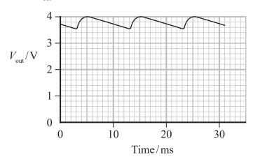
Determine a value for the capacitance of the capacitor.
