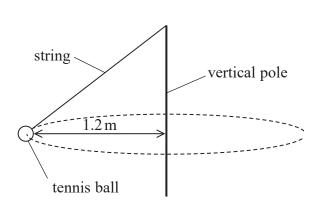
The radius of the path of the ball is  $1.2 \,\mathrm{m}$  and the speed of the ball is  $3.8 \,\mathrm{m\,s^{-1}}$ .
