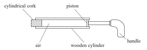
Initially the piston is at the right-hand end of the cylinder, as shown. Then the cork is pushed into the other end of the cylinder.
