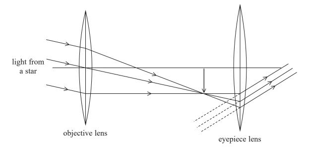
(a) (i) In the arrangement shown, the final image is formed at infinity.
