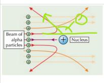
High energy alpha particles were fired into a very thin gold foil. Geiger and Marsden spent days and days recording the angles at which the alpha particles come out of the foil by looking for tiny flashes of light. Mostly the  $\alpha$  particles went through, with some deflection. Very occasionally though a few came back at angles greater than 90 degrees (in green)
