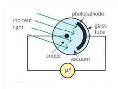
Electrons are emitted at the photocathode by the photoelectric effect. These are then attracted to the anode (why??? - other diagrams on the search engine of your choice show a small cell to create a potential...)
