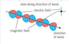
You can see magnetic and electric fields at 90 degrees and in phase. What is really odd is that normally we talk about waves needing a medium to propagate through - ie air for sound, water for ... Well, water waves. E/M waves are able to go through the vacuum of space - ie there appears to be no medium.
