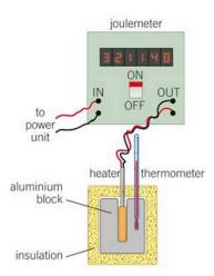
In this practical you have to work out a value for C, the specific heat capacity for an aluminium block.
